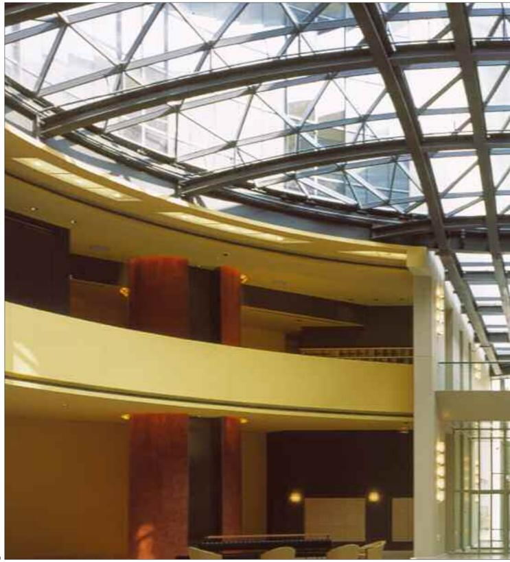
60. The transparent dome is conceived as a system of load-bearing arching girders which support the transverse beams. The longitudinal girders follow the perspective which, starting from the park, projects toward Whitehaven Street.
